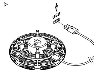
Switch the device off and connect it to a suitable USB port.
